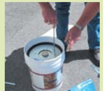
Insert the handle rod into the open nut to remove the follow plate
